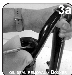
OIL SEAL REMOVAL - BOXXER
