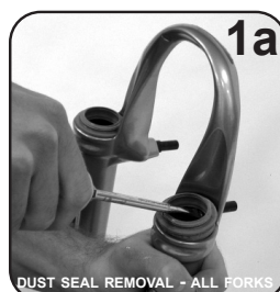
DUST SEAL REMOVAL - ALL FORKS
