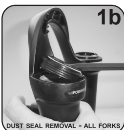
DUST SEAL REMOVAL - ALL FORKS
