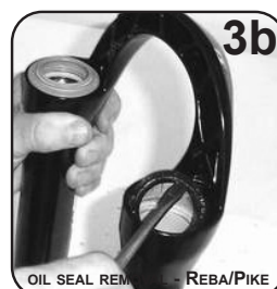
OIL SEAL REMOVAL - REBA/PIKE
